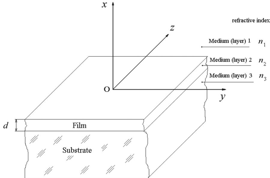
Figure 1: Waveguide is formed by media 1–3. The figure indications are: 1 is a framing medium or cover layer (air) with refractive index  $n_c$ ; 2 is a waveguide layer (film) with a refractive index  $n_f$ ; 3 is a substrate with refractive index  $n_s$ ;  $d$  is the thickness of the waveguide layer. Film and substrate are homogeneous in the  $y$  and  $z$  directions, the substrate is usually much thicker than the film.
