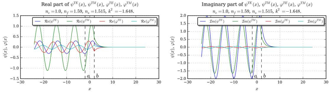
Figure 9: The curves for the field strength (along the vertical axis) for the substrate radiation modes decaying in the cover layer.
