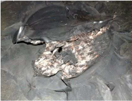
Figure 4: Damage of the conveyor belt-puncture.
