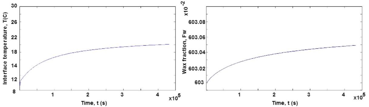
Figure 5: Interface temperature and wax content versus time
