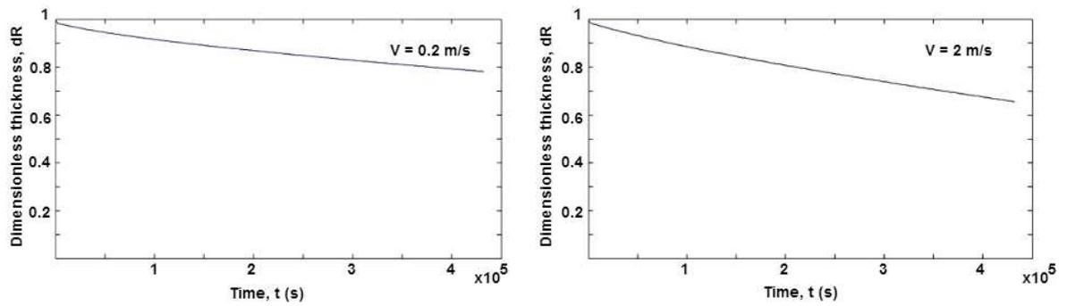
Figure 4: Dimensionless internal radius of the pipe versus time for two values of the flow velocity
