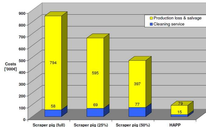
Figure 2: The costs required for procedures of cleaning the pipe with the length 15 km and the paraffin wax layer thickness 10 mm
