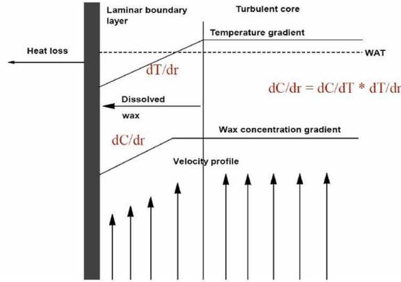
Figure 3: Molecular diffusion as a mechanism of wax deposits forming
