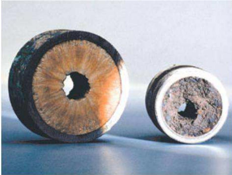
Figure 1: Examples of paraffin deposits in pipelines
